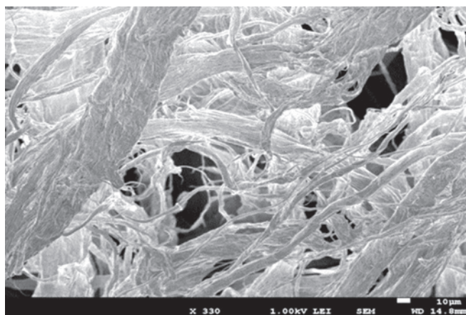
FIGURE 1 ♦ A micrograph of fibrillated HDPE fiber (courtesy of Mitsui Chemicals, Inc.). 3
